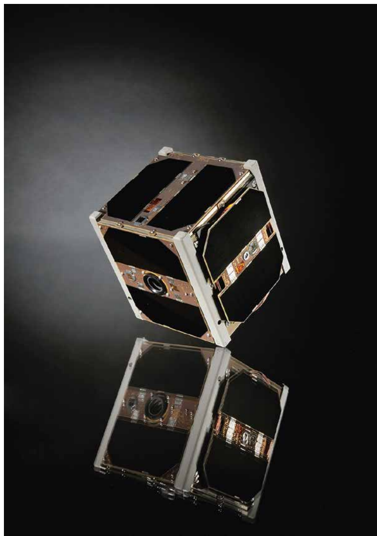
Balancing act: the student built satellite measures just ten centimeters and weighs only 820 grams. Photo: Alain Herzog/EPFL
