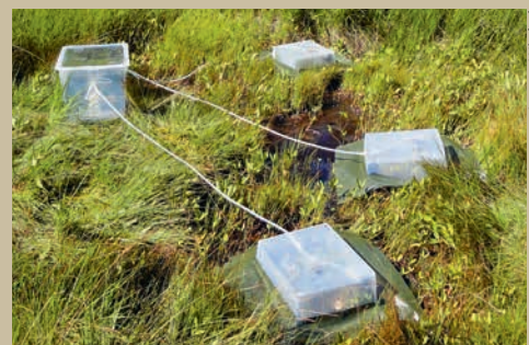
A sulphur trap: setting up an experiment in the Gola di Lago in Ticino.
