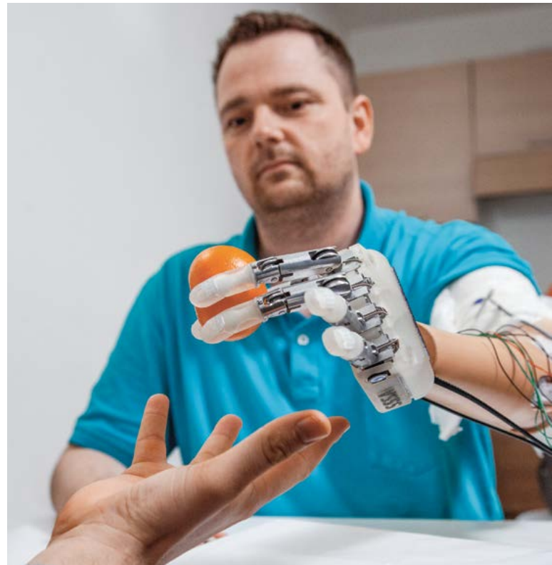
Amputees can control their movements better with a sensory prosthesis that uses an implant to send feedback to the brain.
