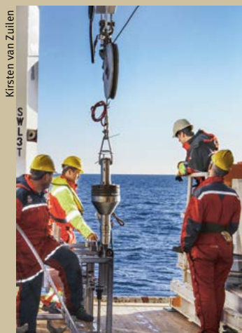
This probe is used to extract sediment samples from the seabed.
