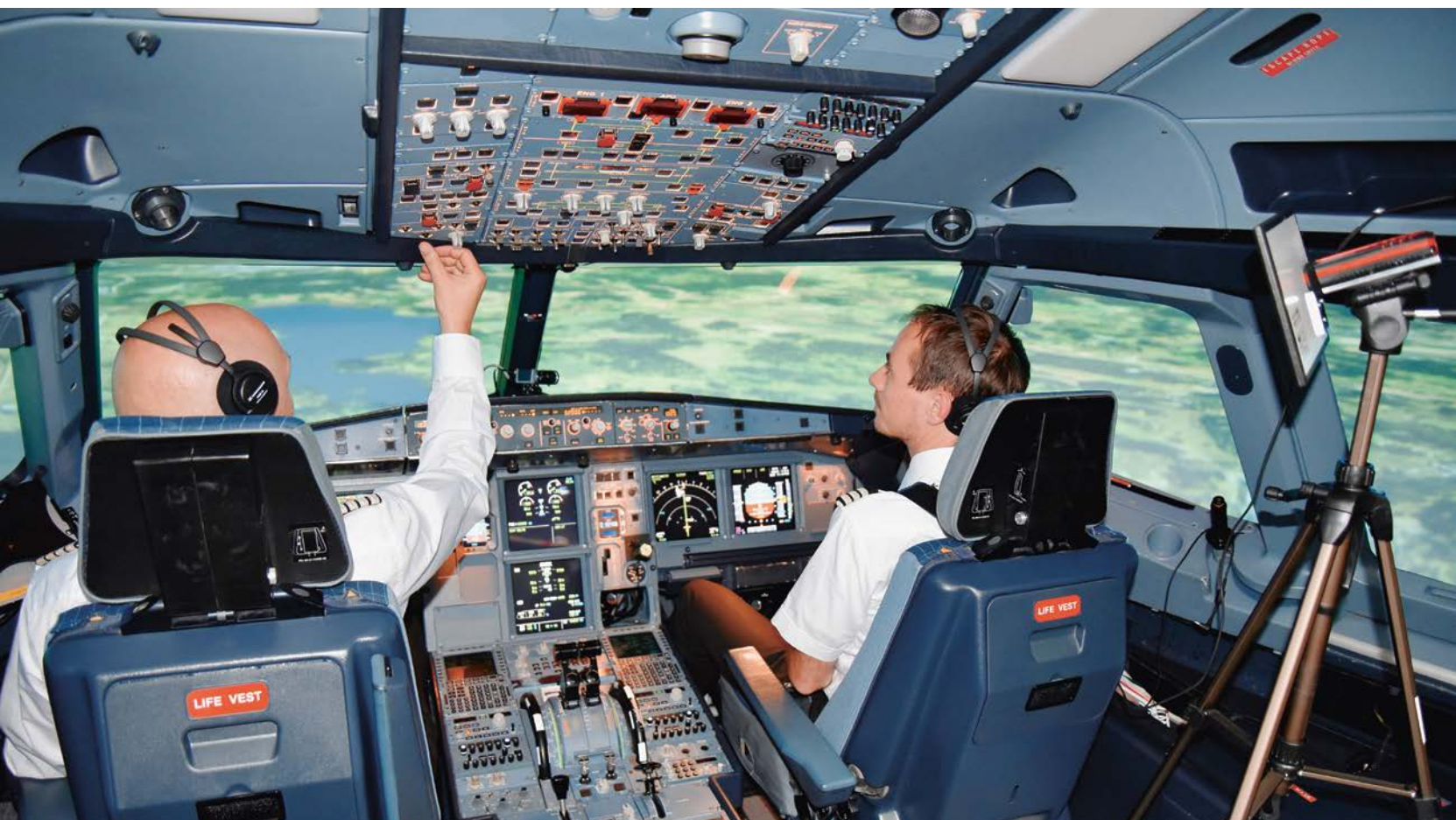
In a flight simulator, infrared flashguns and four cameras help record the gaze of a pilot (left) and his first officer. The combination of flashes and cameras then makes it possible to calculate the direction of vision. Photo: David Rudi
