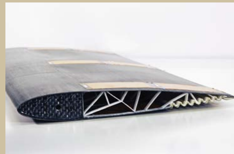
Morphing the end of the wing increases lift considerably and keeps air resistance low.
