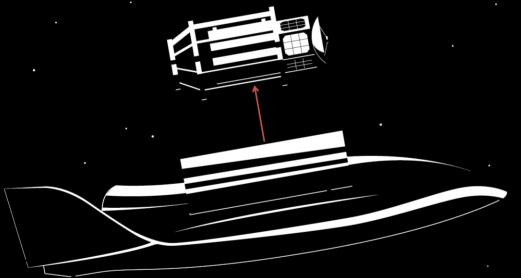
**3** Soar will launch satellites into a low Earth orbit, i.e., a maximum altitude of 700 km. Once detached, its launcher stage will fall back to earth, burning up on re-entry rather than adding to the space clutter that also orbits the Earth.
